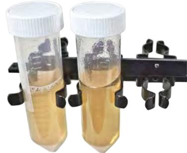
PRS — series platforms are equipped with universal rubber clamps for different size tube fixation;
