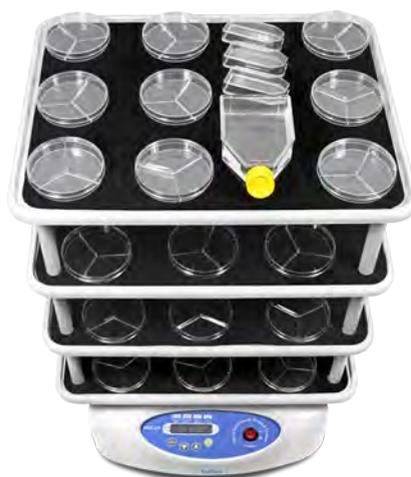
The shaker is designed for application both in small specialised laboratories and in large multidisciplinary laboratories: a choice of nine (9) different interchangeable platforms provides possibility of performing various procedures and techniques. Special attention should be paid to a multilevel platform, which allows accommodation of a large number of various microplates, Petri dishes, cultural bags and other low containers.
