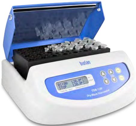
**TDB-120** is a traditional Biosan's dry block thermostat for laboratory analysis. Thermostat is designed for maintaining constant temperature of samples in tubes inserted in the aluminium block sockets. Unprecedented high precision and uniformity of temperature over the block. **TDB-120** is widely used for PCR-analysis.
